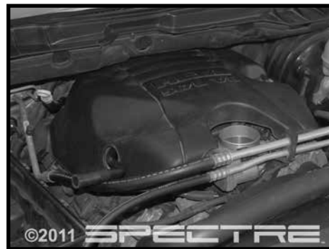
Step 5 Remove the engine cover.
