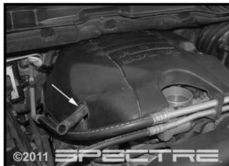
Step 8 Reinstall the engine cover. Make sure the new PCV breather line fits into notch on the engine cover.
