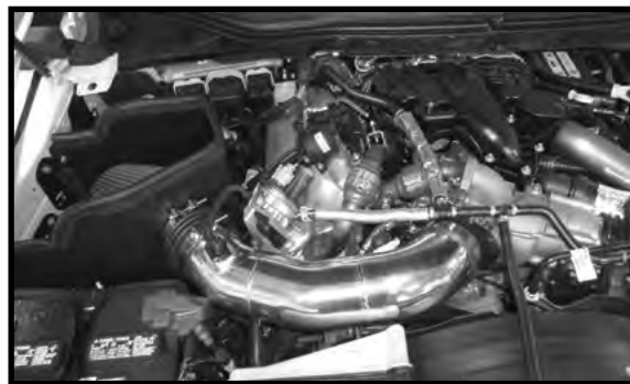
Step 20 Make sure that all clamps and hardware are fully tightened. Reconnect the battery cable, start the vehicle and let it warm up. Shut off and inspect the installation once more for any loose clamps, wires, or hardware. Test drive & enjoy! Your installation is now complete. Periodically check all clamps and brackets.
