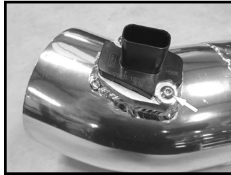
Step 18 Install MAF sensor into Spectre air intake tube with provided bolts.
