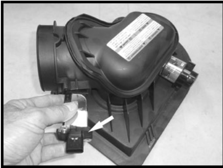
Step 17 Remove MAF sensor from factory air box.
