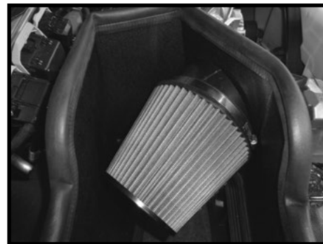
Step 15 Install air filter. Clock so filter has clearance on all sides.
