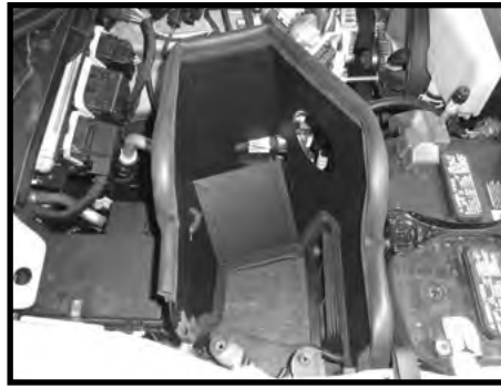
Step 9 Install heatshield into vehicle as shown.
