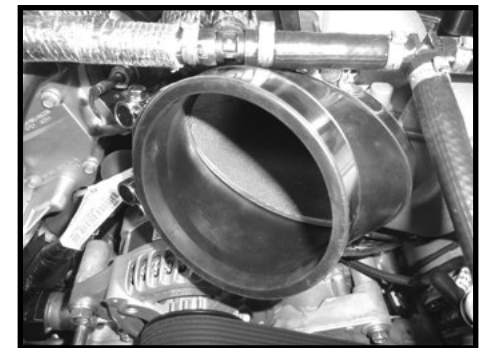
Step 16 Install intake manifold coupler and tighten one clamp.
