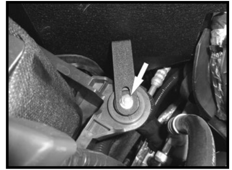
Step 10 Install outer L bracket with nylon mounting stud as shown.
