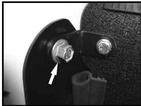
Step 11 Install upper L bracket with bolt removed in step 5.
