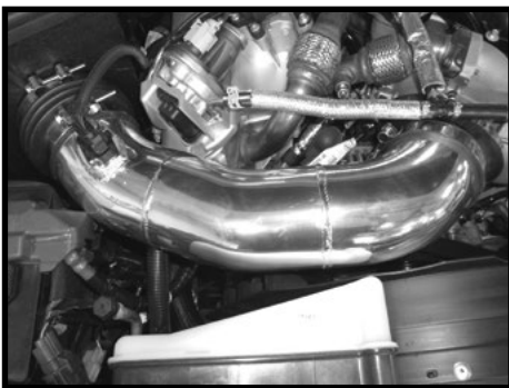
Step 19 Install intake tube, Align and tighten clamps. Install MAF sensor extension cable attach to factory wiring harness. Make sure it does not interfere with any moving parts.
