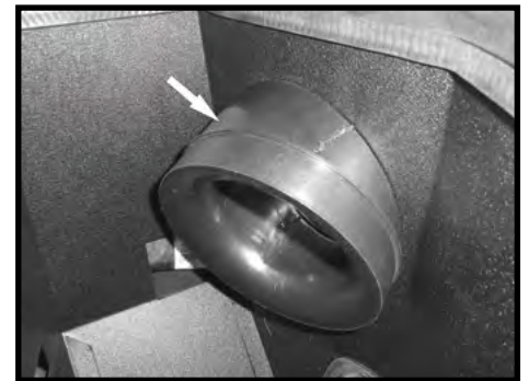
Step 13 Install air filter velocity funnel in heatshield.
