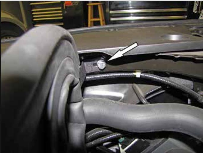
7. Secure the front of the heat shield to the core support with the provided hardware as shown.
