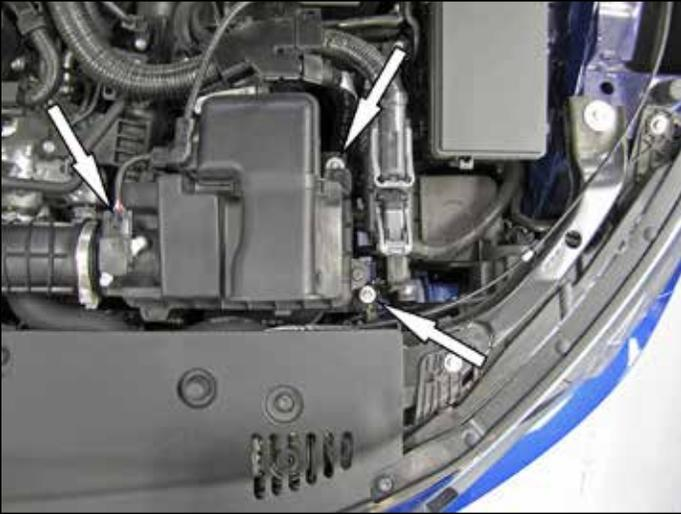
2. Disconnect the mass air sensor electrical connection. Remove the two bolts that secure the factory air filter housing.
