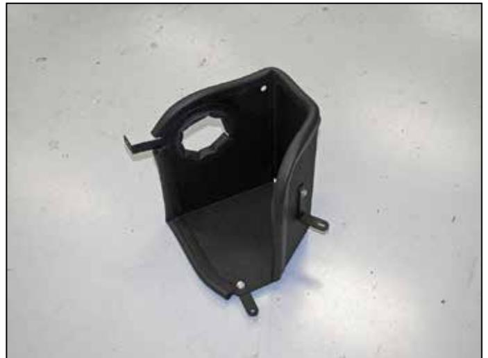
5. Install the provided heat shield mounting brackets and edge trim onto the heat shield as shown.
