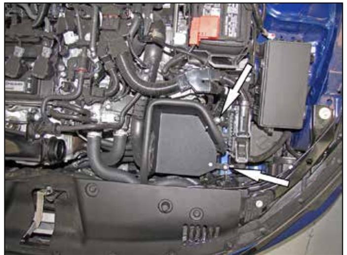
6. Install the heat shield assembly into the vehicle and secure with the provided hardware where shown.
