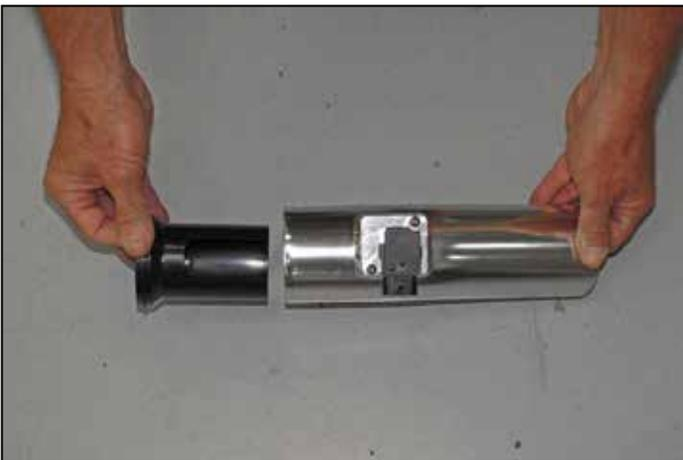
9. Remove the mass air sensor from the factory intake system and then install it into the SPECTRE® intake tube. Install the maf sleeve into the intake tube as shown, the sleeve should slide all the way in until the lip contacts the end of the tube.
