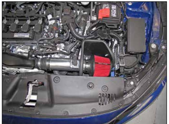
12. Reconnect the maf sensor electrical connection.
