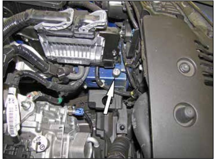
4. Install the provided rubber mounted stud into the inner fender where shown.
