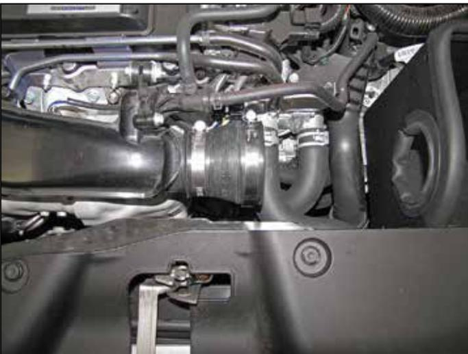
8. Install the provided step coupler onto the turbo inlet and secure with the provided hose clamp.
