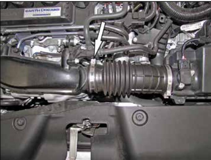
3. Loosen the hose clamp that secures the factory intake tube to the turbo inlet pipe. Lift up and remove the complete intake system.
