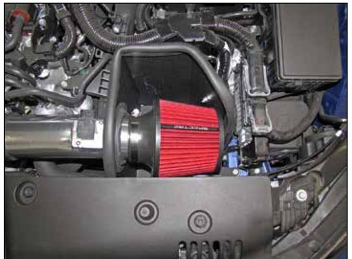
11. Install the SPECTRE® air filter onto the intake tube and secure with the provided hose clamp.
