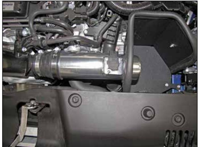
10. Install the SPECTRE® intake tube into the heat shield and then into the coupler hose, adjust for best fit and then secure with the provided hose clamp.
