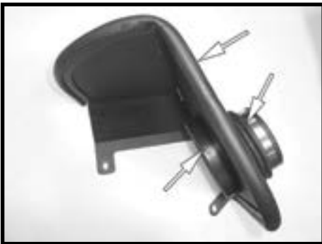
Step 10 Assemble the heat shield with the tabs placed on the outside of heat shield. Install the rubber bulb seal, this may require trimming to the correct length. Place the velocity stack adapter in the heat shield and install the supplied flex coupler making sure the coupler is pushed completely against the heat shield. Take note of the orientation of the funnel, this may be rotated slightly once the filter is installed in the vehicle. Once the adapter and coupler are tight against the heat shield, tighten the clamp.
