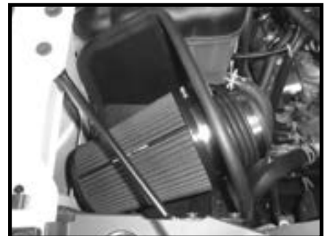
Step 14 Install the filter and fully tighten the clamp. Rotate the bracket back into position and reinstall the bolt removed in the previous step.
